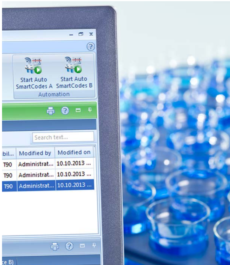
Figure 9: The SmartCodes function of LabX permits users to link titration methods directly to samples, such that sequential samples need not be analyzed using the same protocol.
