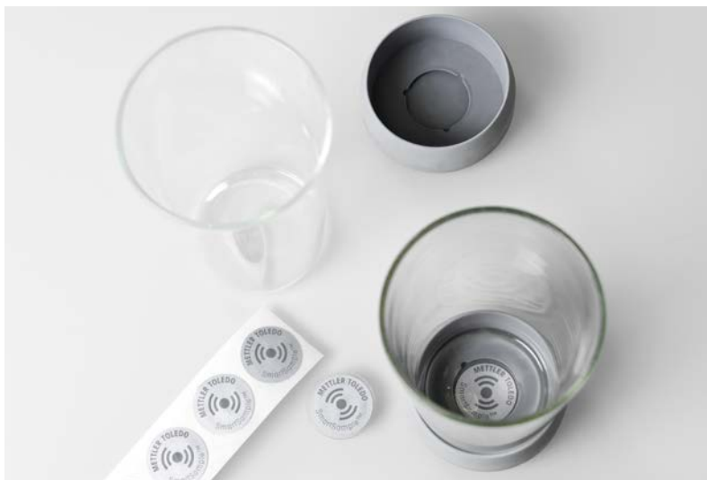
Figure 8: RFID-enabled Smart Tags attach to sample beakers, linking each titration sample's data and metadata to it from the balance to the results.
