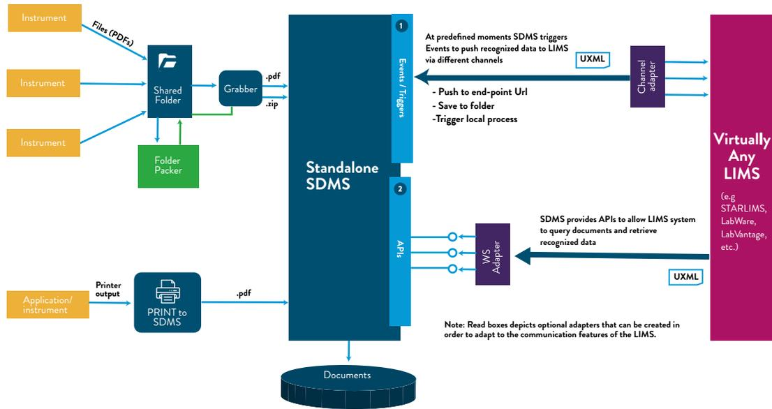
Figure 2: Methods for interconnecting STARLIMS SDMS
