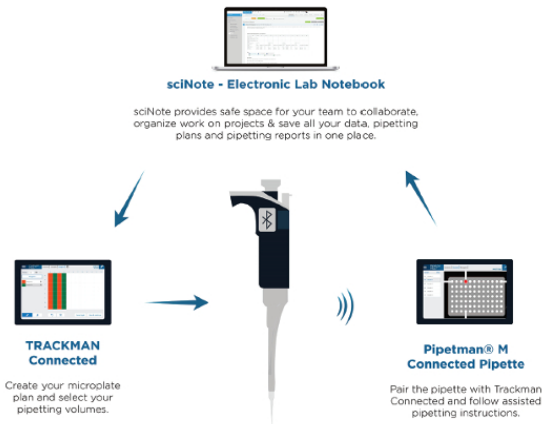
Figure 1 – Cloud-enabled pipetting and data recording. A pipetting plan can be created using a microplate tracker application, which collects data on each pipette stroke by Bluetooth pairing to a smart pipette. This will help researchers detect manual errors that occur during an experiment. After the pipetting is done, a detailed pipetting report can be saved in an electronic lab notebook and reused later as a template for the next experiment. (Source: Gilson, Inc. and sciNote.)
